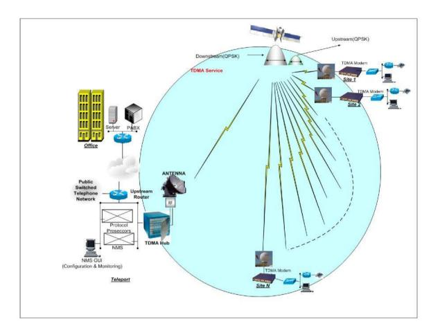
TDMA VSAT service may include installation and configuration of equipment to transmit and receive data over satellite. The service does not include Customer Premise Equipment (CPE) needed to terminate the signals - these can be purchased or leased separately.
