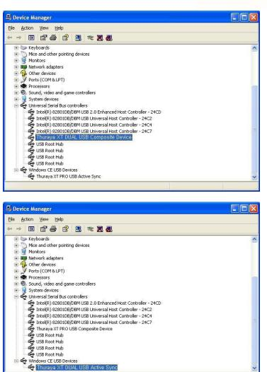
Thuraya XT DUAL USB Composite Device is now installed under 'Universal Serial Bus controllers' and Thuraya XT DUAL Active Sync is now installed under 'Windows CE USB Devices'.
