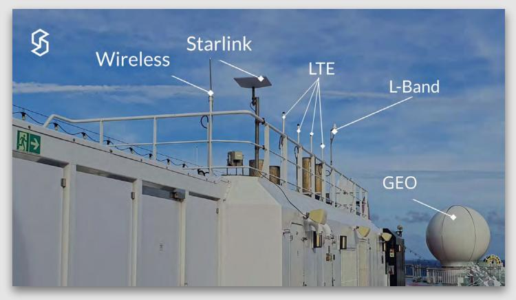
which operate in polar regions and three in Europe, we're using C and Ku-band GEO and Starlink, doing load balancing and bonding the satellite links with Talari SD-WAN and managing them with Speedcast Truebeam.
